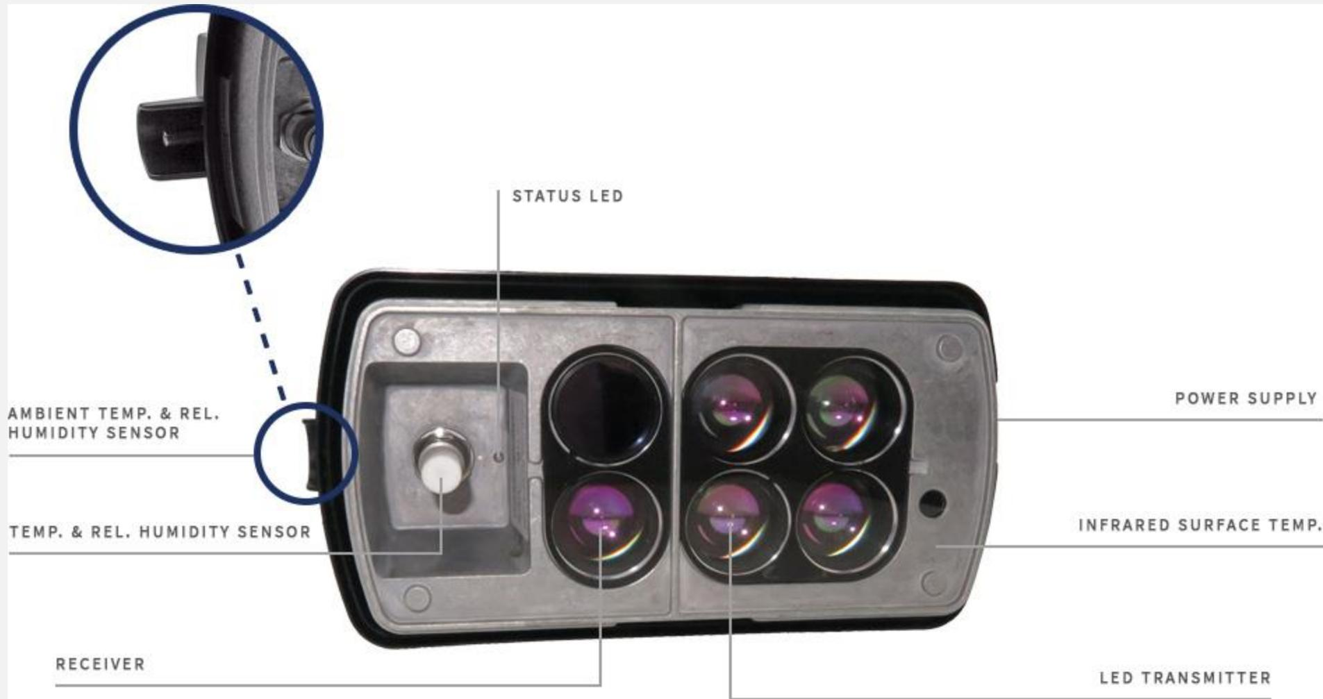
**MARWIS delivers the following data:** Road surface temperature, waterfilm height, dew point temperature; road conditions: dry, moist, wet, snow, ice; ice percentage; friction; rel. humidity, air temperature
