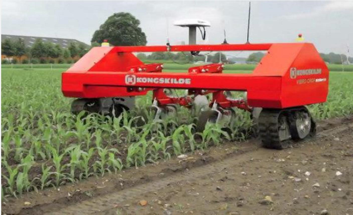
It can be equipped with Vibro Crop Intelli sections for mechanical weed control or implements for precision seeding (Becker Aeromat or Centra), ridging discs and mechanical row crop cleaning units (Kongskilde Vibro Crop). -
