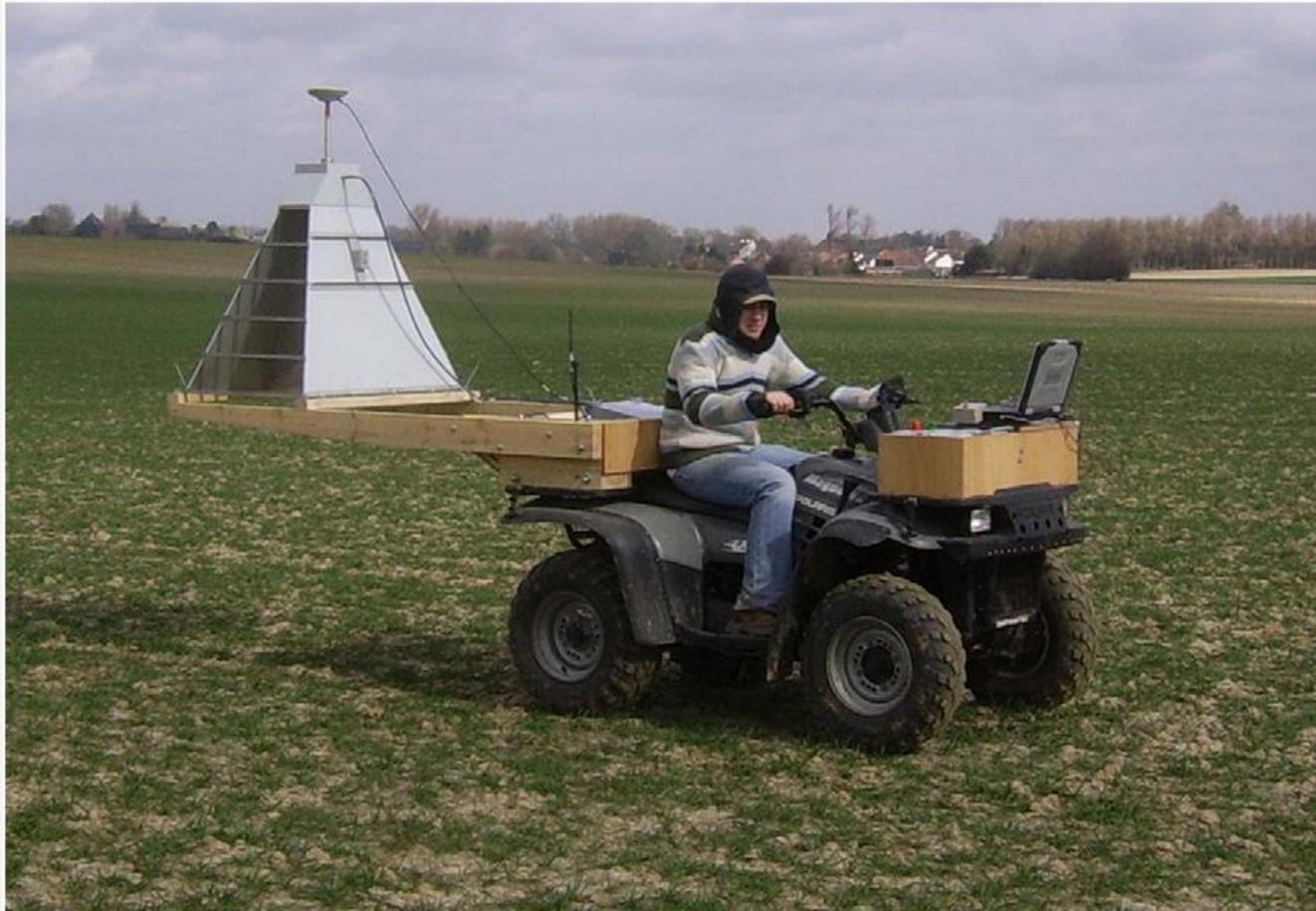
Four-wheel motorcycle holding the GPR system constituted of a horn antenna linked to a vector network analyzer, the DGPS device and the laptop.
