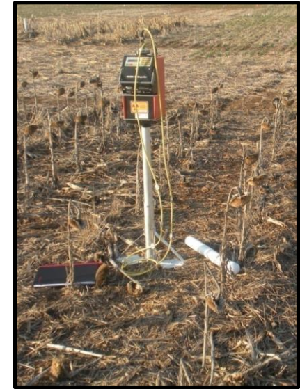
Neutron probe depths: 10, 30, 50,...,190 cm.
