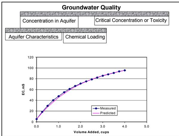
The simple experiment utilizes portable electrical conductivity meters as an indirect measure of salt concentration in the inflowing water and in the “aquifer”. This demonstrates that the simple model can describe concentration changes in the idealized aquifer.
